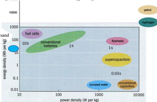
Figure 2. Characteristics of selected energy storage schemes
